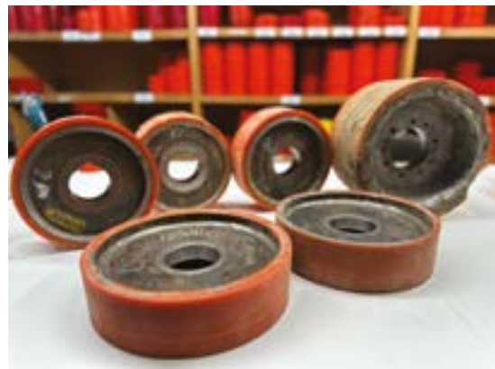
Planer and Rip Hubs pre-recovering process.
